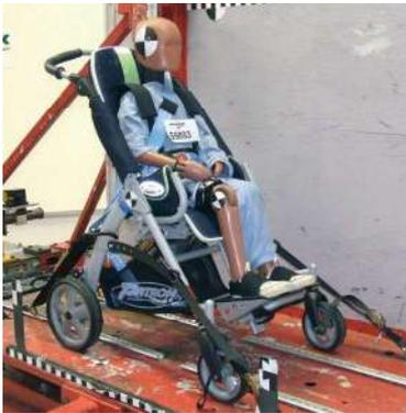
The product had been successfully crash tested and fulfilled all the requirements of EN ISO 7176/19. It enables to use the rehab-buggy not only for a common duty, but as well as for the transportation in specially adjusted motor vehicles, equipped with the anchoring points and equipment.
