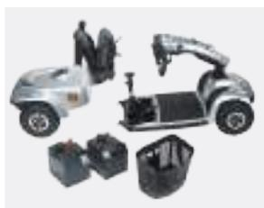
Disassembly into five parts
